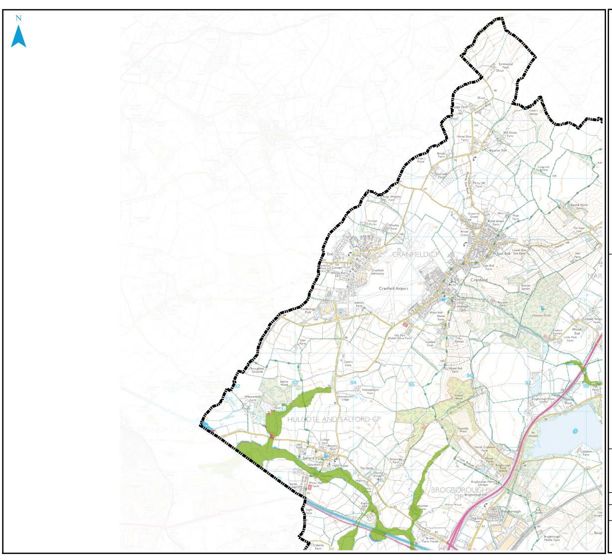
Outside of the detailed model extents, where Flood Zones are still present, Jflow modelling has been undertaken, applying the relevant change factor to the 100-year flows.
