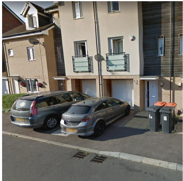
Leaving half a car length in front of a garage results in vehicles parking and over-hanging the footway, particularly when one garage is the only form of parking provided.
