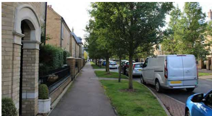
Figure 191: Careful siting of trees and using suitable species is important so that it does not obstruct visibility, Fairfield
